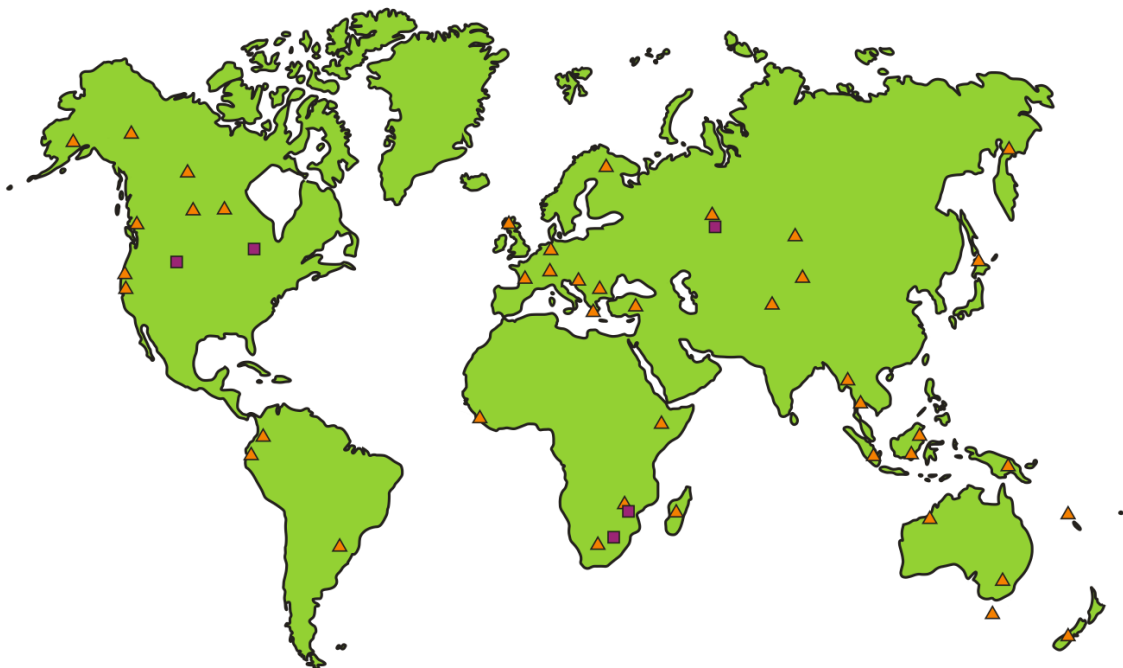
Figure 1. 1 Global distribution of PGM placers (orange triangles) and significant PGE-bearing stratiform complexes (purple squares). After Weiser (2002).
