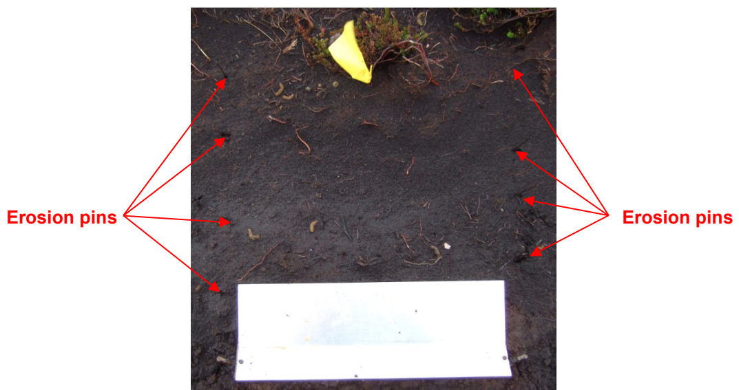
Figure 3.7: The set-up of a monitoring framework to assess the sediment transfer from slopes. The Gerlach trough is located at the foot of the slope while the arrangement of 8 erosion pins (two sets of 4 pins in a vertical array) is also visible. The width of the trough is 0.5 m.
