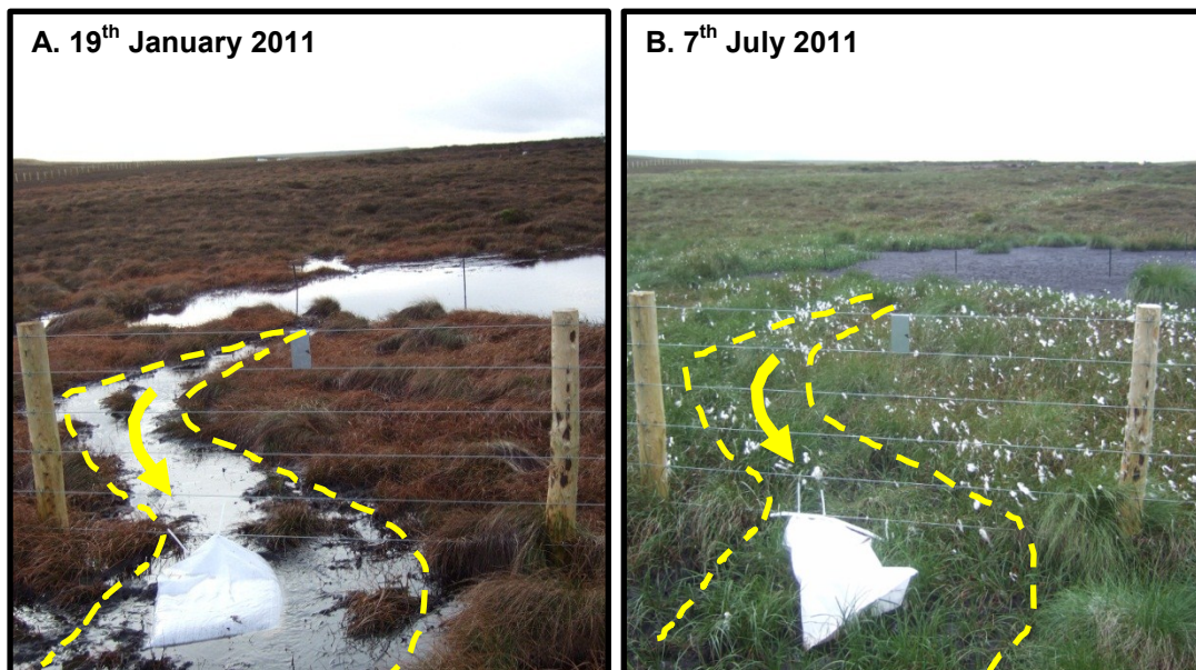
Figure 4.18: Channel draining depositional pool monitored by sack trap number 3 A. Photo taken on 19 th January 2011 B. 7 th July 2011. By July, vegetation has grown in the channel, trapping sediment and preventing the loss of peat from the site.
