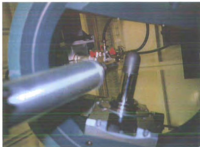
Figure 4.7 A view of evacuated incoming photon tube, sample holder and cryostat at BM28.
