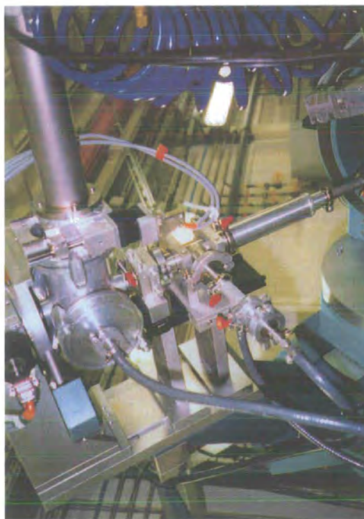
Figure 4.8 A view of evacuated scattered beam tube, analyser crystal stage and detector in BM28.
