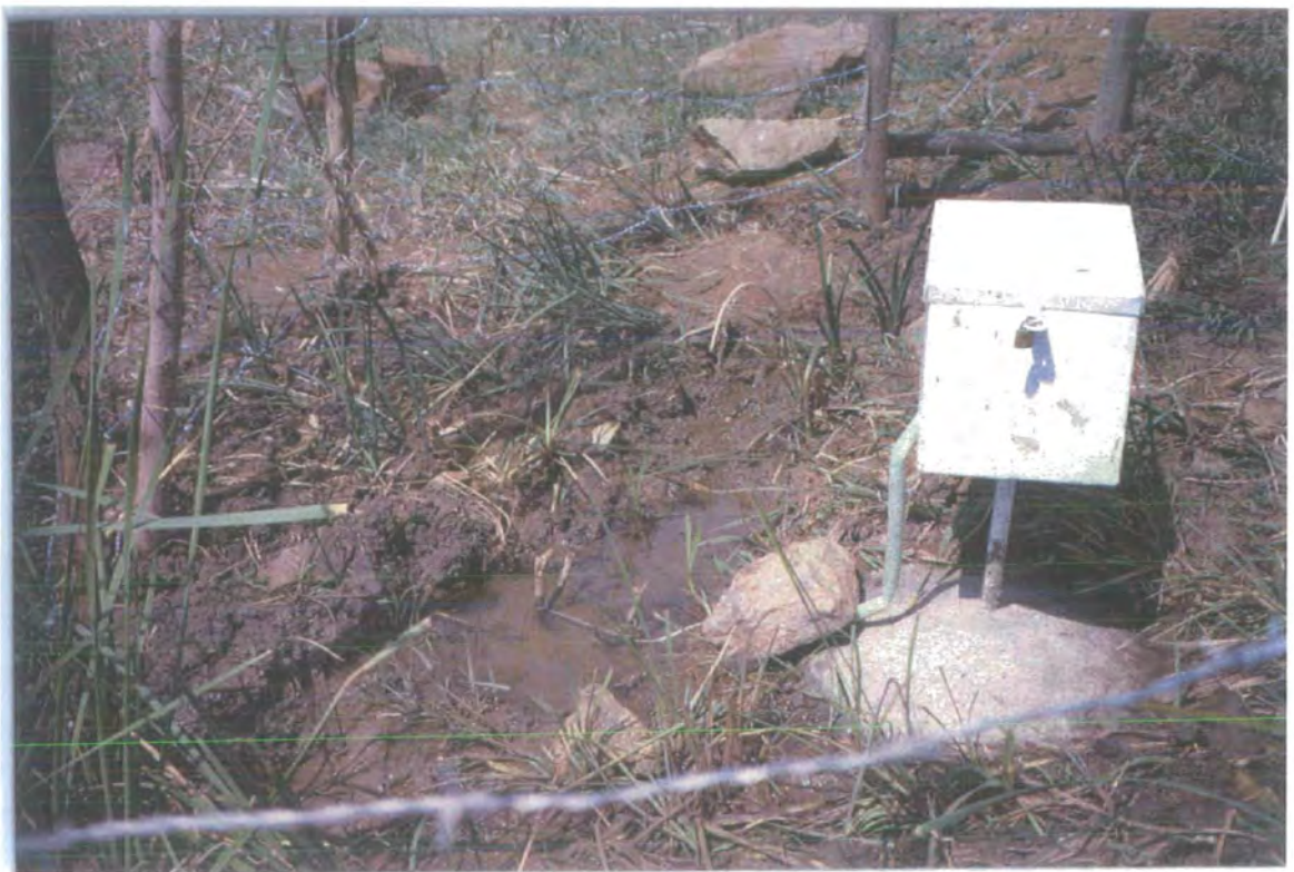
Plate 3.3. A temperature probe in seepage water (data logger inside the white box)
