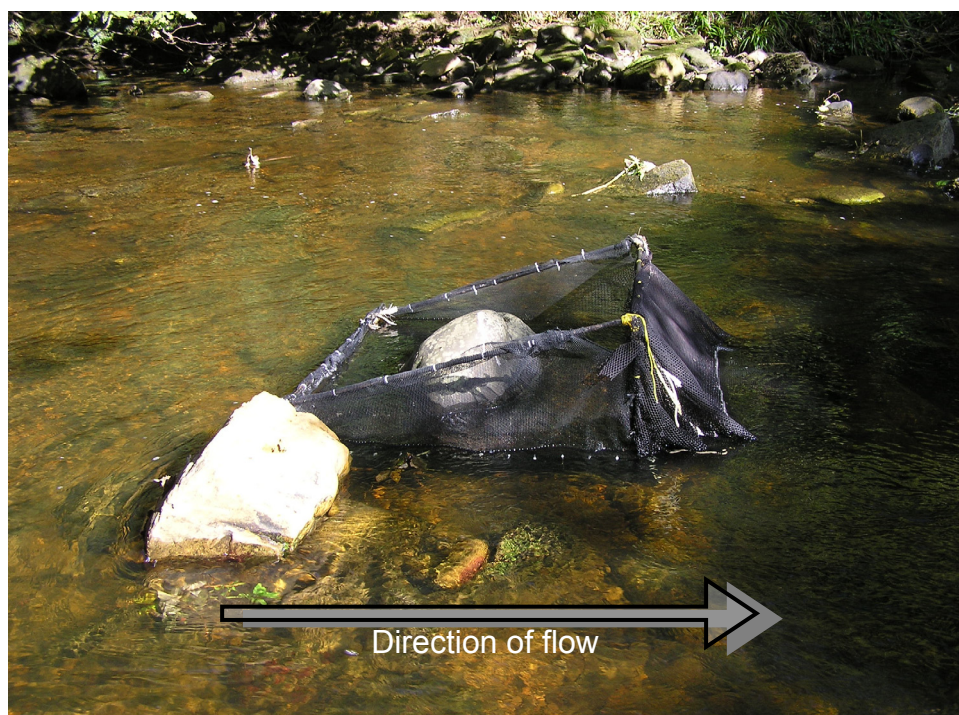
Figure 2.2- Photograph of the Surber sampler used to capture crayfish and delimit the area for microhabitat recording
