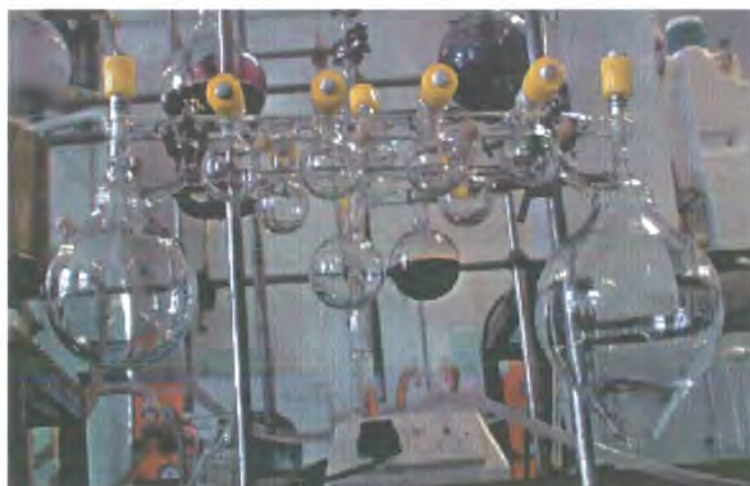
Figure 23: The multi-flask reaction vessel used for star synthesis.
