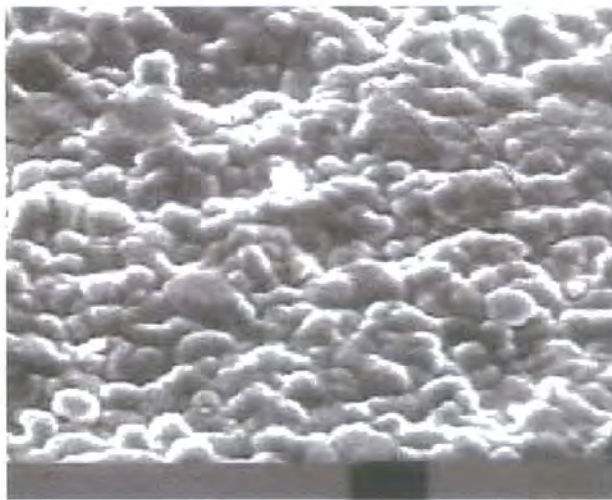
Fig. 3.21 E-beam evaporated film on Al 2 O 3 , annealed at 500°C
