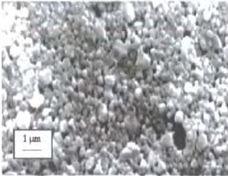
Fig. 4.13 SEM image for a film with glass phase, fired at 850°C for 30 min
