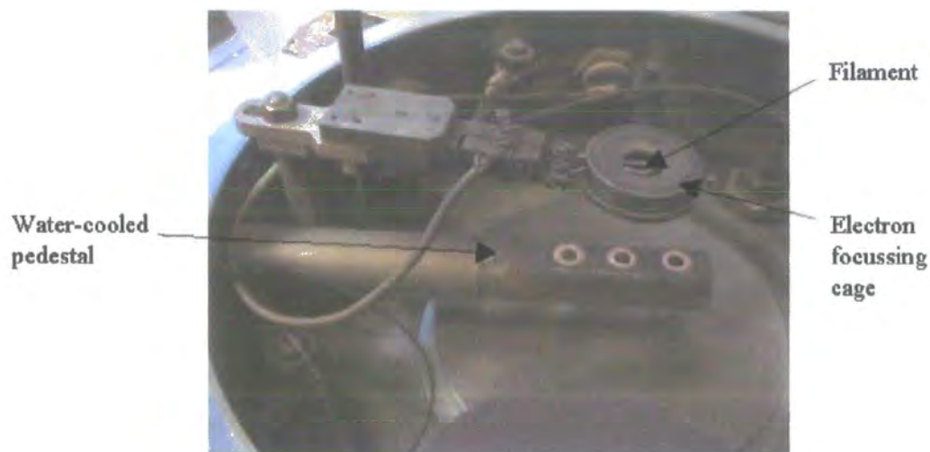
Fig. 3.4 Electron-beam source assembly
