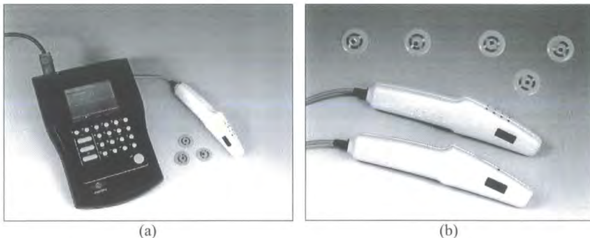
Figure 2.4 Proximity reader developed for safety test market. Slide (a): portable appliance tester (right) and proximity reader (left). Slide (b): two proximity reader models shown with low-frequency transponders. Components are manufactured by Seaward Electronic Ltd., including transponder assembly.
