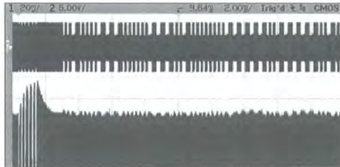
Figure 10.8 Digital demodulation of the sampled RF carrier. Top trace: Transponder terminal voltage, showing load modulation of the field. Bottom trace: Base band signal recovered by rectification in digital domain.
