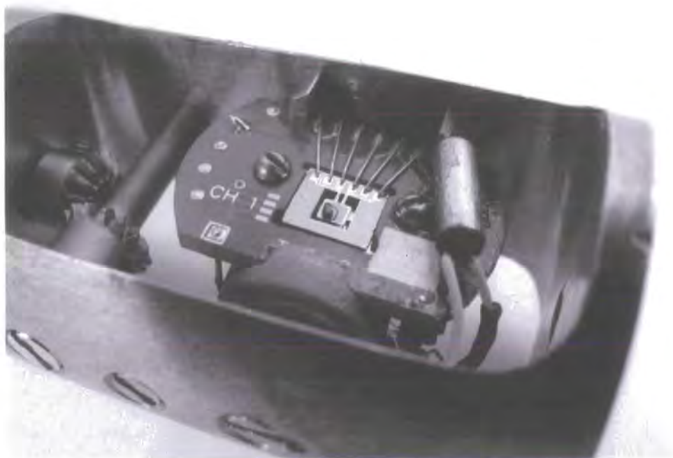
Figure 5.5. Photograph of the field-gradient torque magnetometer copper cage end piece, with the rotational set-up inside. The QD torque chip is in the centre of the tufnol chip holder. The sample on the platform is \text{Pb}_{0.75}\text{Eu}_{0.25}\text{Mo}_6\text{S}_8 , and is glued on using GE varnish.
