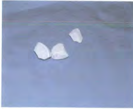
Figure 3.12 Photograph of the aluminium PolyHIPE composite.
