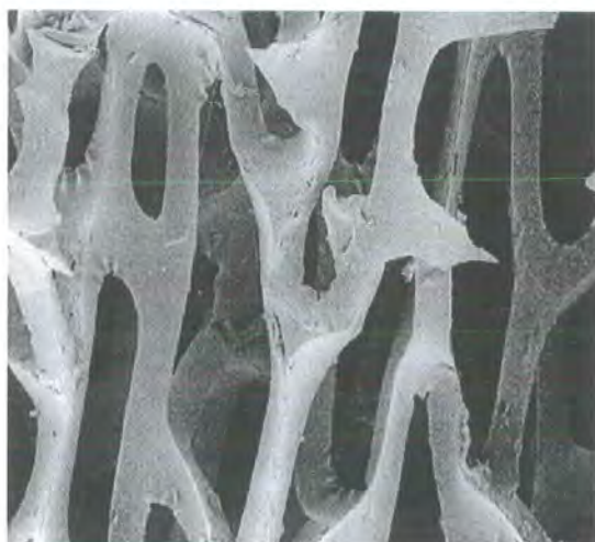
Figure 10.1 SEM image of a polyurethane foam with anisotropic structure and Poisson's ratio greater than 1 (151) .
