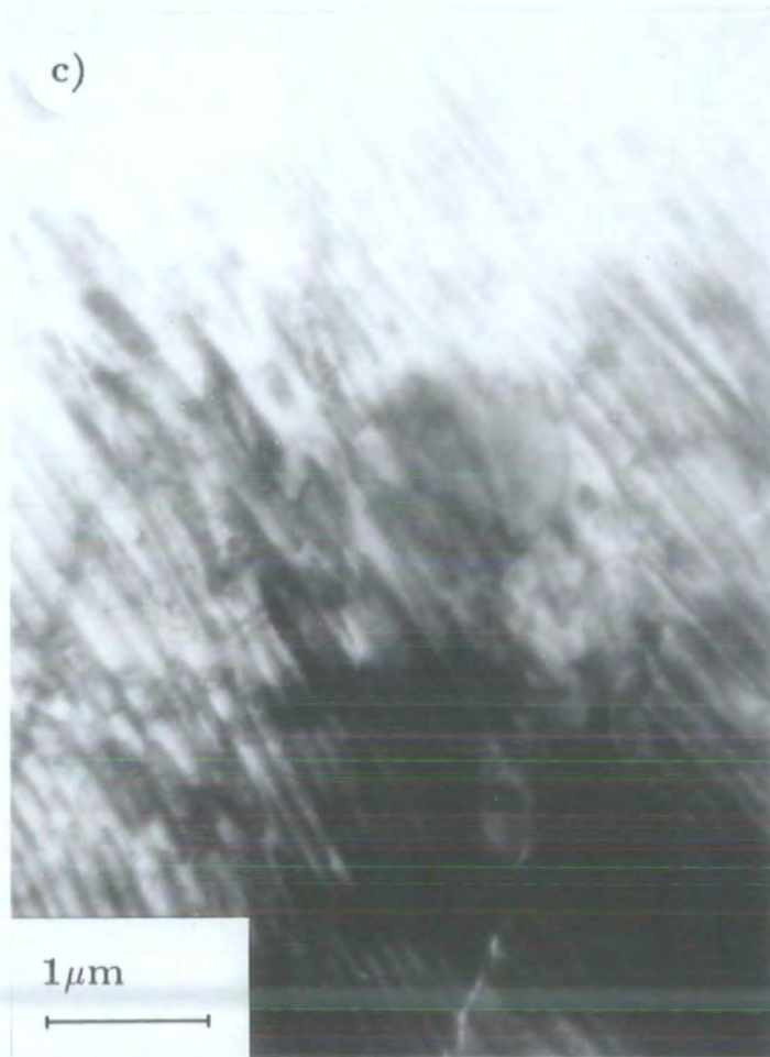
Figure 4.21 Fresnel electron micrographs of undeformed 2401 pipe steel : a) infocus, b) underfocus, c) overfocus.
