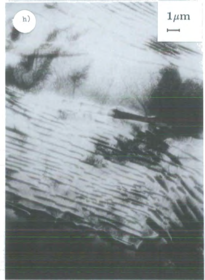
Figure 5.44 contd. e) underfocus after removing the field, f) underfocus at -2\text{kAm}^{-1} , g) underfocus at -8.3\text{kAm}^{-1} and h) after removing the negative field.
