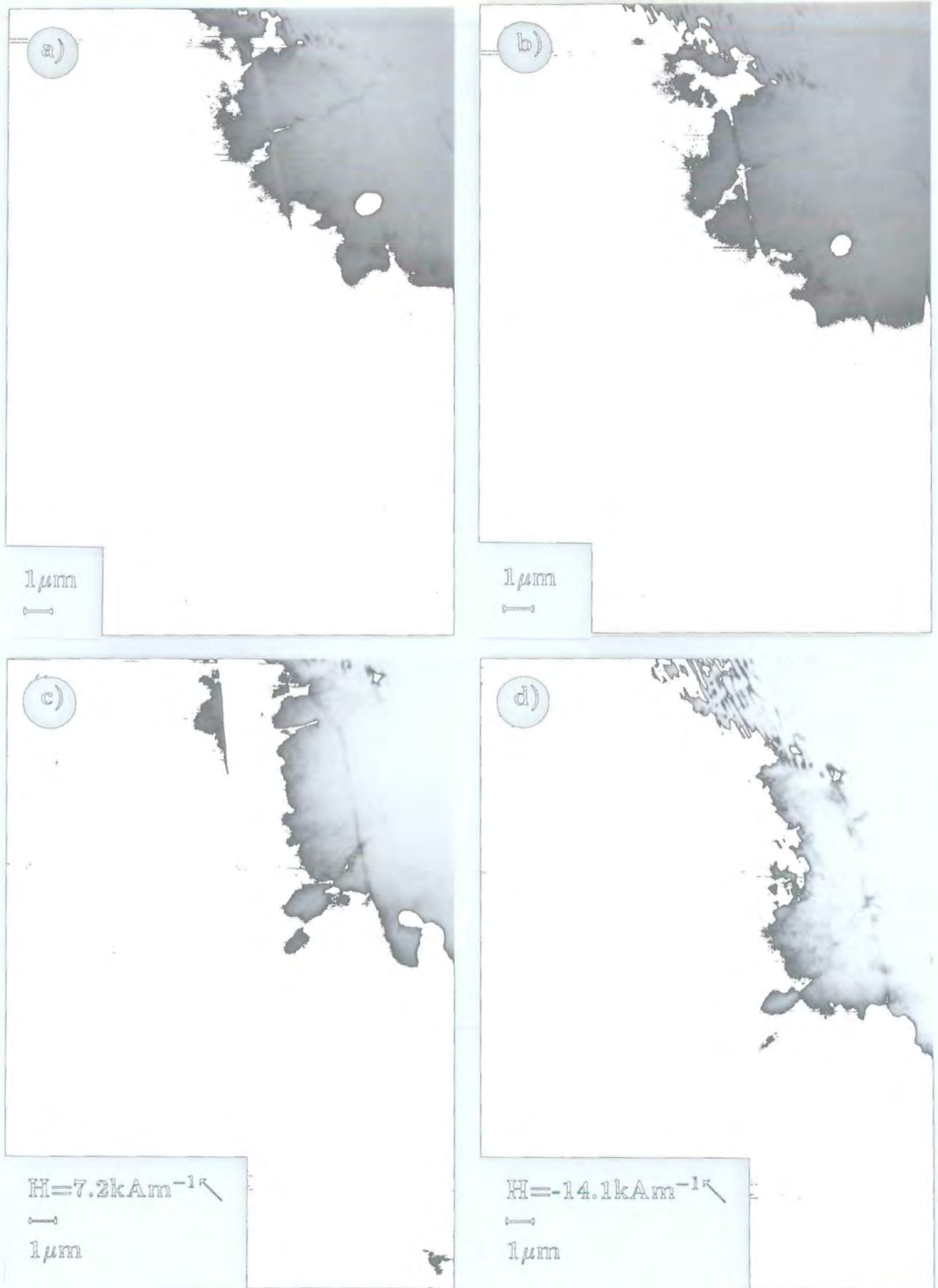
Figure 5.33 Fresnel electron micrographs of undeformed 7092 : a) infocus, b) underfocus, c) underfocus, at 7.2\text{kAm}^{-1} and d) underfocus after reducing to -14.1\text{kAm}^{-1} .
