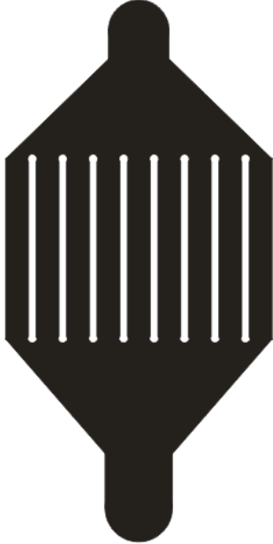
Fig. 83. SU8-50 microfluidic channels mask.
