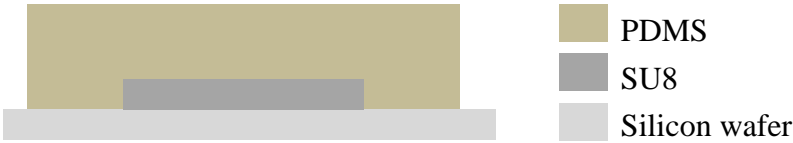
Fig. 85. Cross section diagram of the SU8 mould covered with liquid PDMS.
