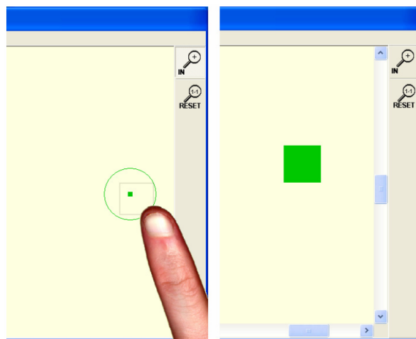
Figure 2.7 – The ‘Zoom-Pointing’ method. The user zooms to a sub area defined by drawing a rectangle (left). The user can then perform direct pointing at a finer scale (right). (Albinsson and Zhai, 2003).
