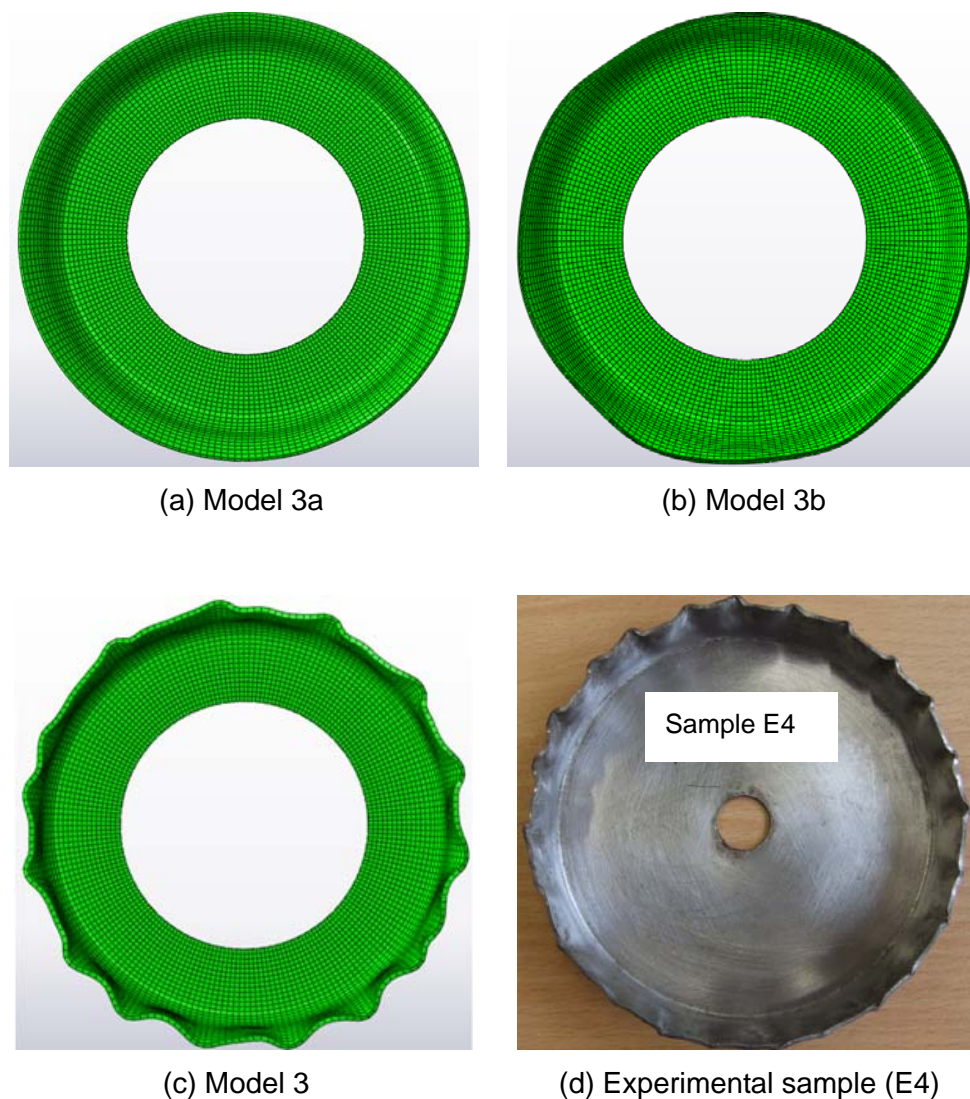
Figure 6.5 Comparison of deformed workpiece using different types and numbers of elements
