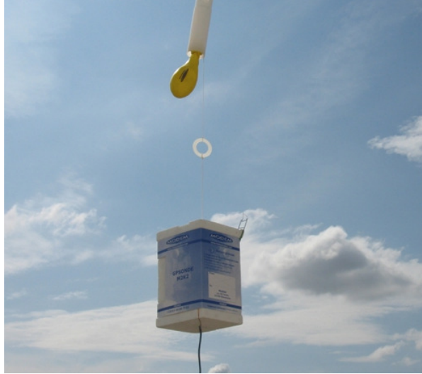
Figure 4.2: Photograph of a thermosonde and the boom. The boom is located about 10 meters below to avoid disturbances from the balloon.
