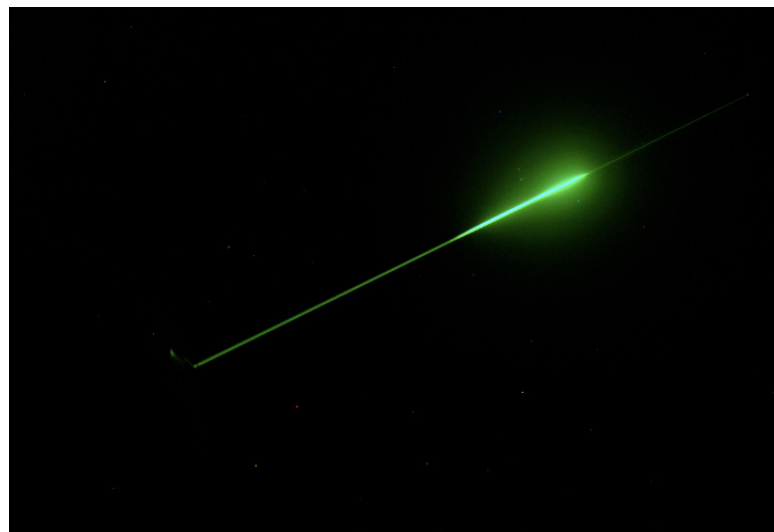
Figure D.8: Laser Guide Star scatter due to an event of dust. Credit. Juan Carlos Guerra
