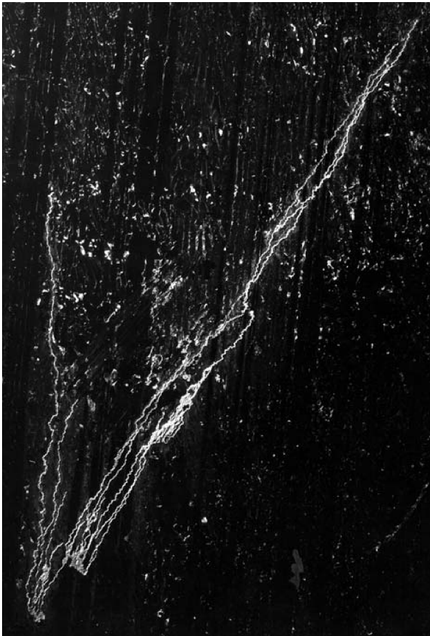
Fig. 9 Photograph of a coreplate showing an unusual interlaminar breakdown in a large hydrogen-cooled turbogenerator subjected to a core fault, as described in [19]
