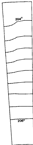
Fig.6. FE calculation of temperature rise on the ring outer surface at 10s. Only the left hand side part of the ring segment is shown.
