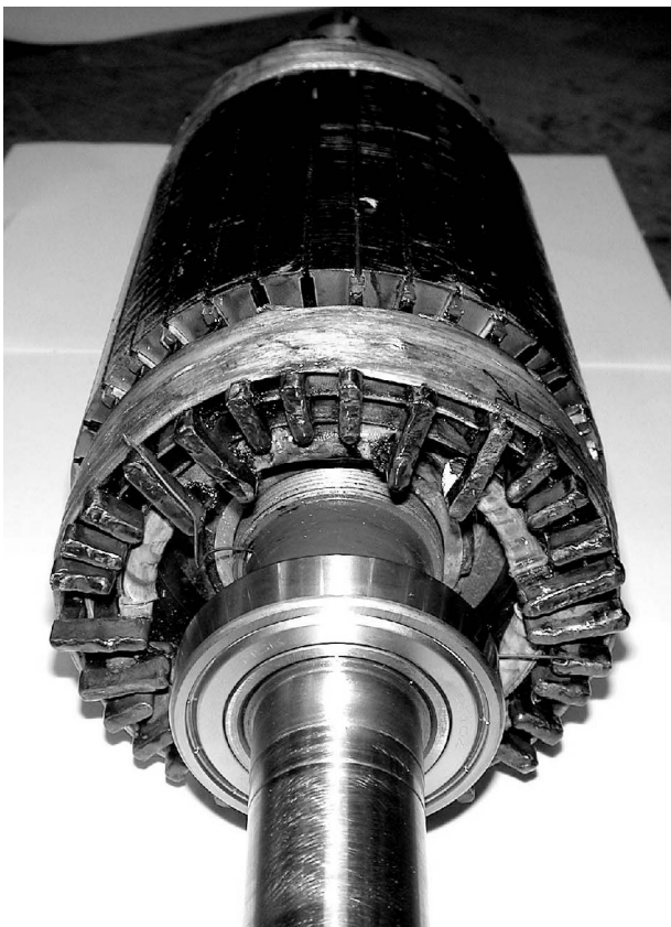
Fig. 3 Rotor 3: Prototype new double layer design
