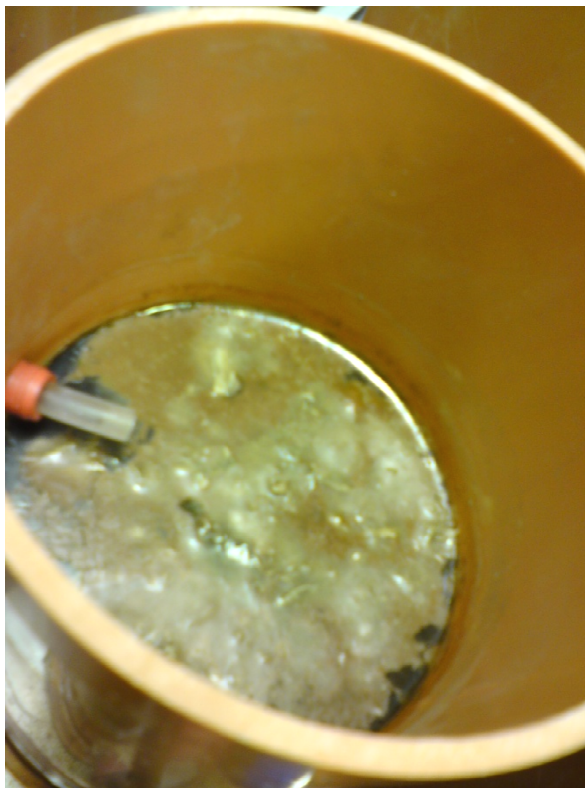
Figure 6.3: Microbial/Fe film developed over waterlogged sample.
