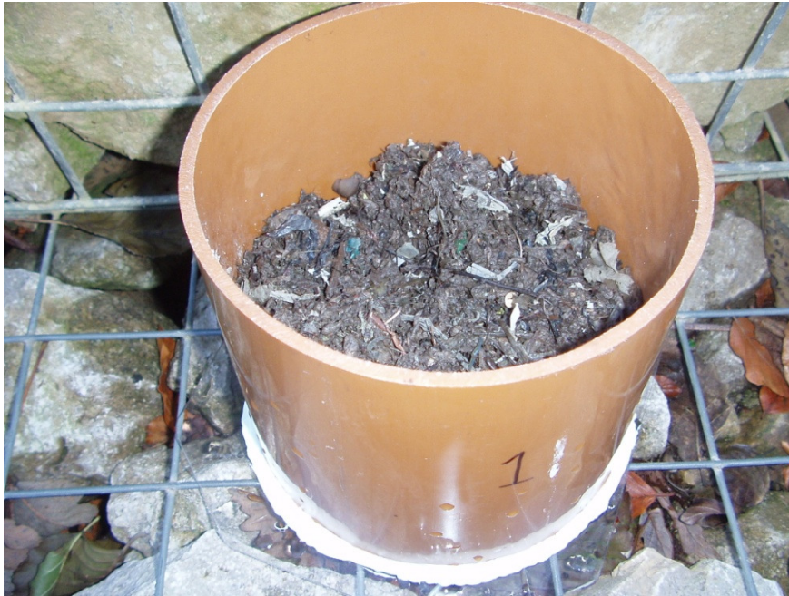
Figure 3.2: Lysimeter used in trial 1
