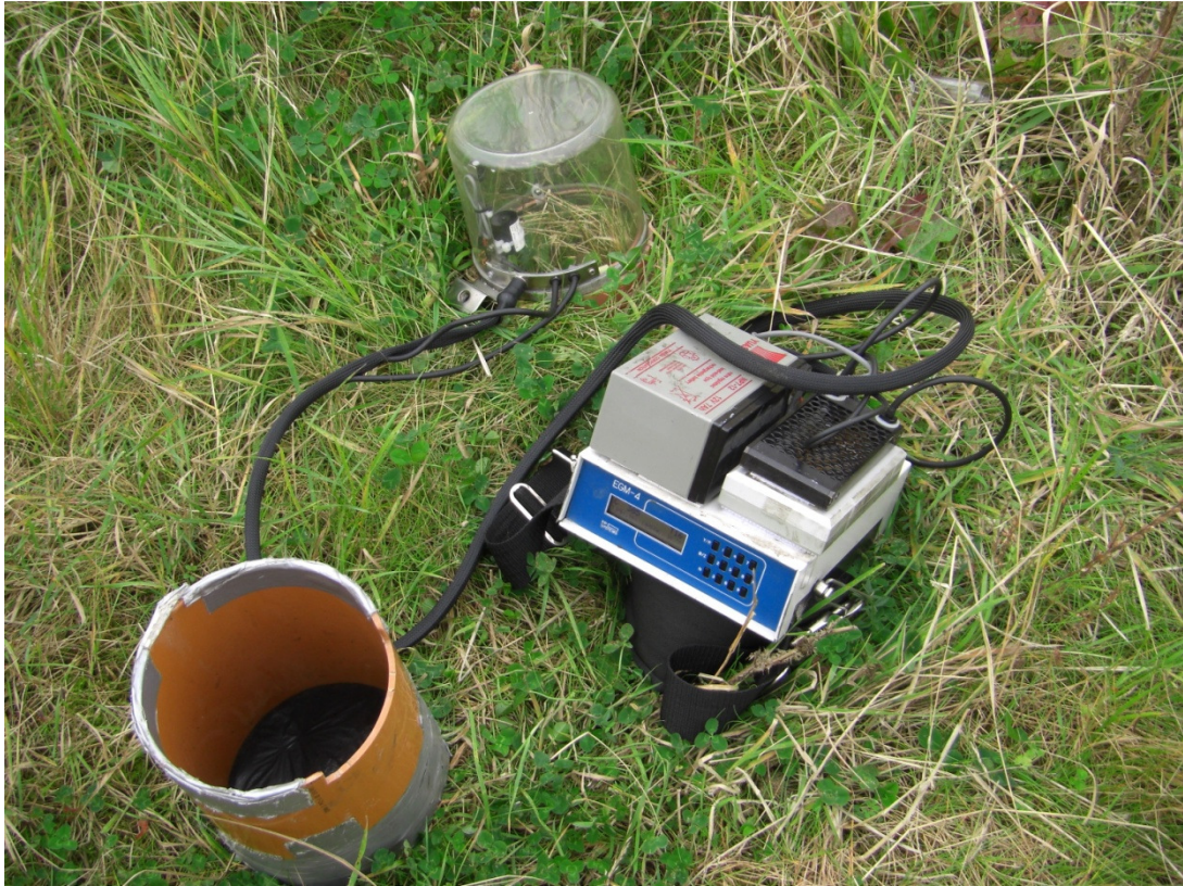
Figure 3.3: EGM-4 Environmental Gas Monitor with canopy chamber. The piping is used as a hood to eliminate any photosynthetic effects.
