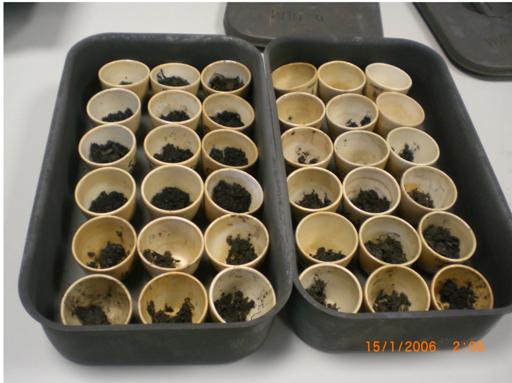
Figure 5.1: Photograph of two of the metal trays, each containing 18 PTGA samples in labelled, ceramic crucibles.
