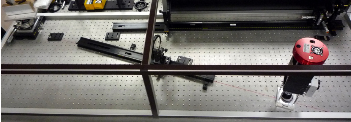
Figure 6.4: The spectrograph test-bench used for experimental investigations. For reasons of measurement stability the entire setup is enclosed by a light tight box (the metal frame supporting the structure can be seen on the picture).
