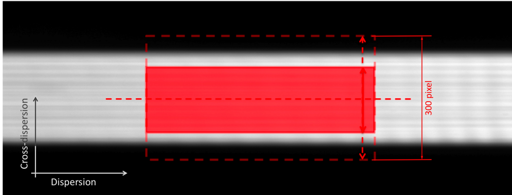
Figure 6.12: The scheme is depicted for which different integration ranges are chosen in order to derive the optimum value for the number of rows to be included for further analysis. All integration ranges are central to the axis.
