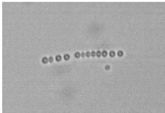
Figure 4.8: Line array of 620 nm PS at \lambda = 880 nm, in p -pol. A group of five particles is seen to be clustered together and appear ellipsoidal. The most closely spaced particles are only 620 nm apart, and are possibly squeezed out of the trapping plane in the z -direction. ( n_{BK7} = 1.507 ; \theta_c = 62.2^\circ ; \theta_i = 64.5^\circ )
