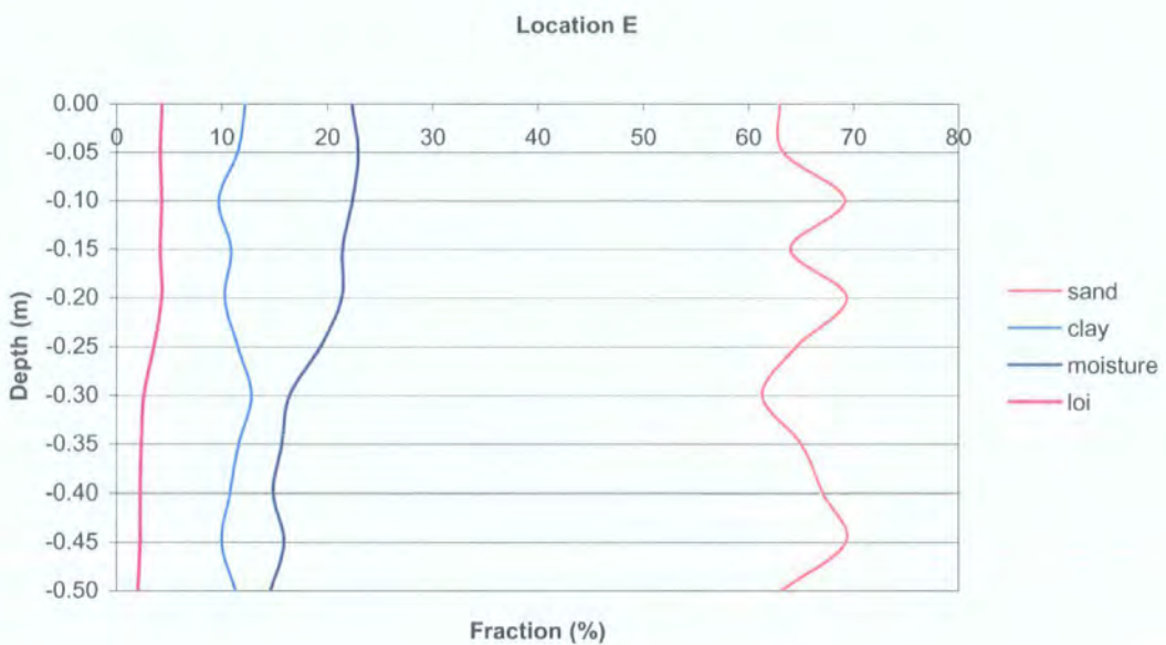
Figure 7.29: Vertical soil profile extracted from Bosworth Location E
