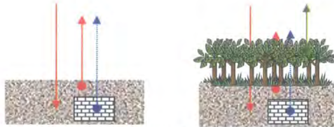
Figure 3.4: Effect of vegetation on thermal response detected at the surface
