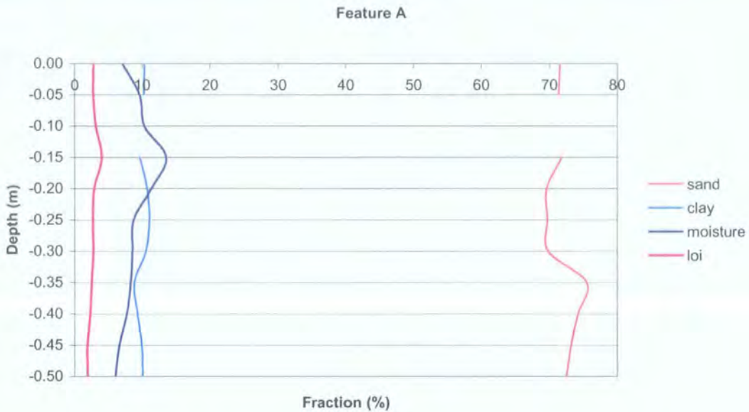
Figure 7.25: Vertical soil profile extracted from Bosworth Feature A
