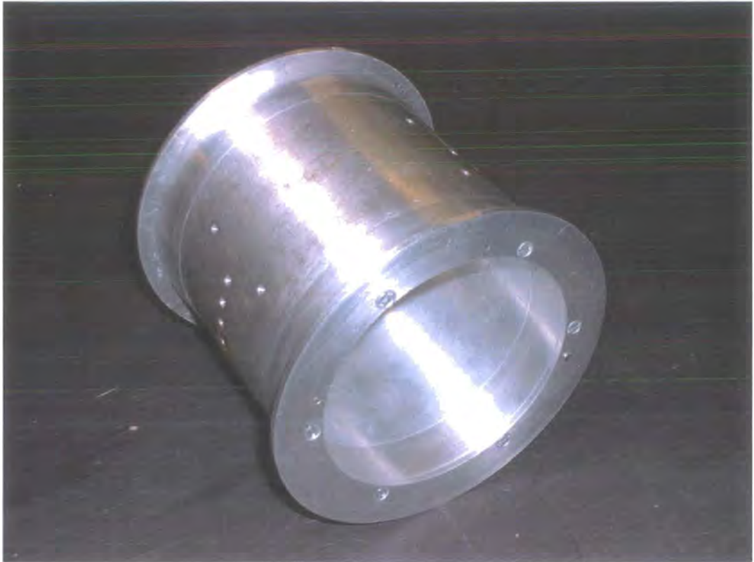
Figure 3.3: The Assembled Multi-Element Wheel Rim Assembly.
