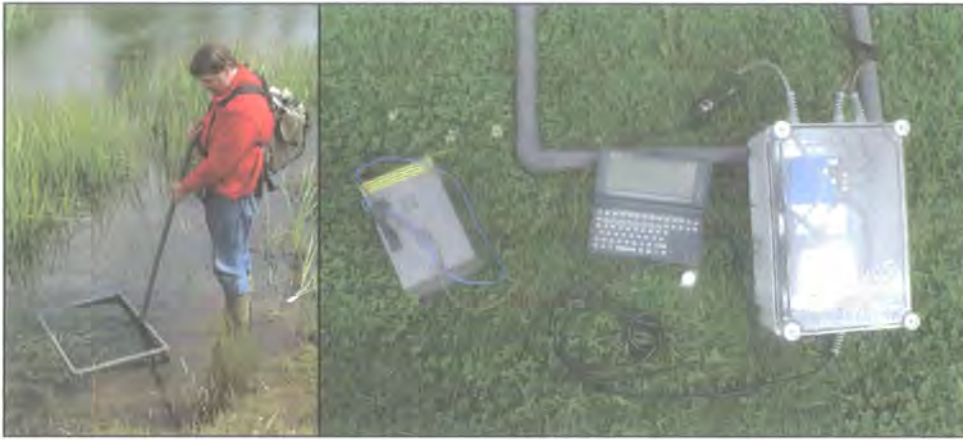
Figure 3.2 a) Portable 23-mm PIT reader in use b) the rechargeable 12-V battery, palmtop computer and reader and control module (viewed from left to right).
