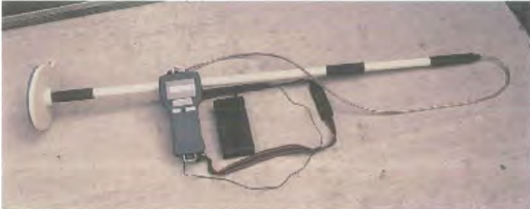
Figure 3.1 Prototype 12-mm Passive Integrated Transponder (PIT) tag reader (UKID Systems, Preston, UK), shown with external battery pack (black casing). Pole with search head measures 1.5 m.
