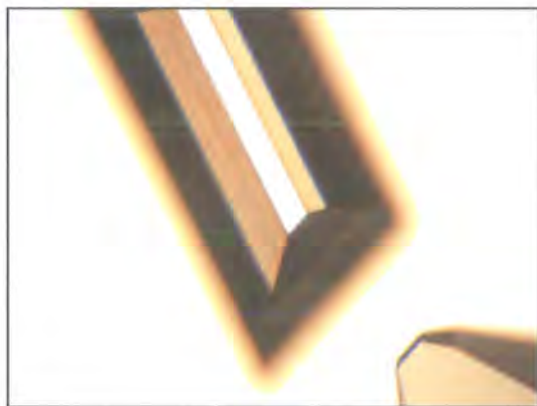
Figure 5.8. Glycine crystal grown under a monolayer of 2-aminohexadecanoic acid viewed with high magnification. Scale : 1\text{ cm} = 50\ \mu\text{m} .
