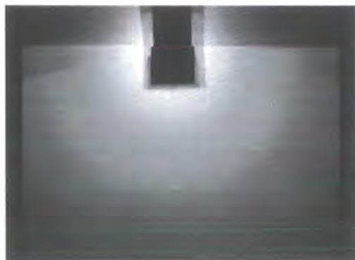
Figure 3.24. Image plate taken with sample lowered out of the beam path, showing subtle features due to background and mylar film.
