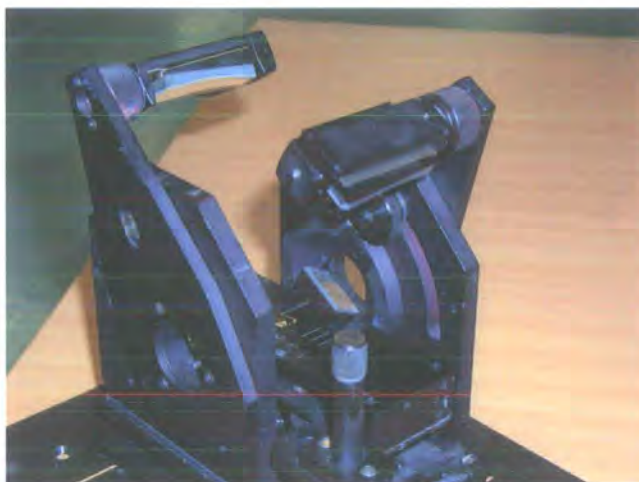
Figure 2.8. Image of Spec-Ac external reflectance accessory. The concave mirrors and the planar mirror after the source are visible.
