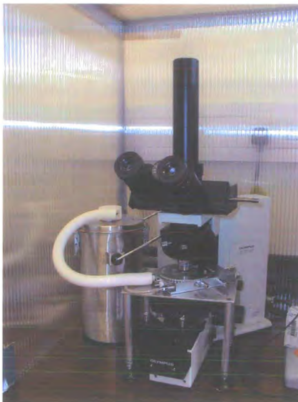
Figure 2.6. Image of optical microscope, equipped with Linkam controlled temperature stage.
