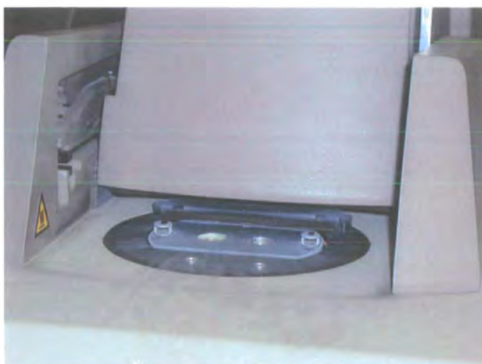
Figure 4.4. Picture of sample environment in the DSC instrument.
