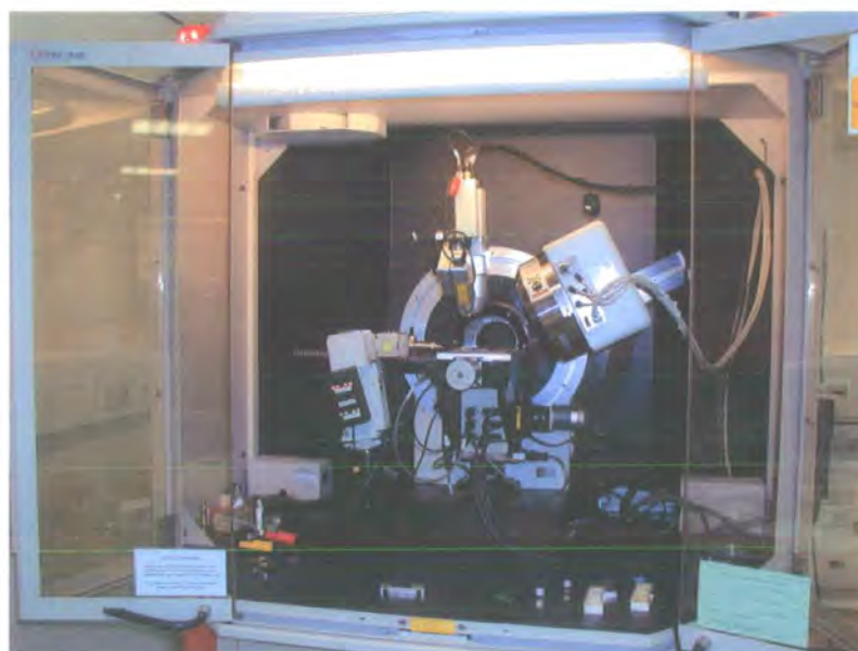
Figure 3.14. Picture of Bruker D8 WAX diffractometer.
