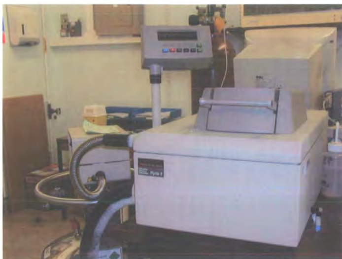
Figure 4.3. Image of Perkin Elmer Pyris 1 DSC. The liquid nitrogen dewar required for the sub-ambient temperature studies detailed in this chapter is visible at the bottom left of the image.
