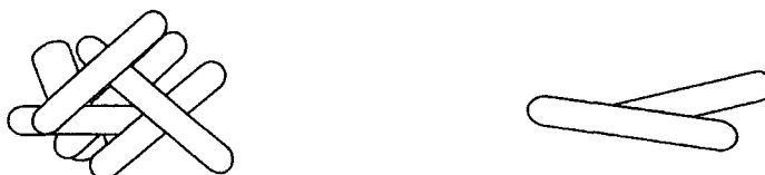
Figure 4-24. Large cluster with small or no anisotropy (left); small cluster with high anisotropy (right)
