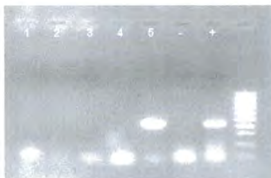
Figure III.13 BSA titration for a forensic sample. Lanes 1-5 are decreasing concentrations of BSA: 0.32, 0.24, 0.16, 0.12 and 0.08 \mu\text{g}/\mu\text{l} , respectively.
