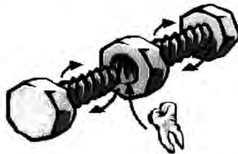
Figure III.3 Scheme of the nut & bolt apparatus. The tooth is placed inside the nut and then the bolt screwed in so that the dental sample breaks.
