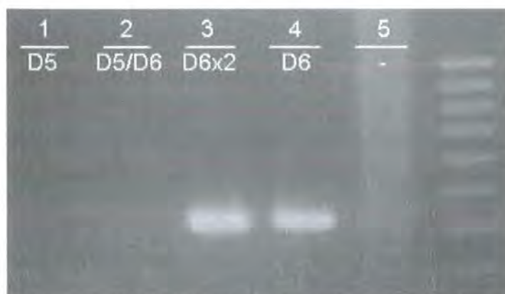
Figure III.10 Lack of amplification reaction due to inhibitory compounds. Lanes 1 to 4 show the amplification results of 25 \mu l-PCR mixes for: (1) 5 \mu l of forensic sample D5, thought to present inhibitory compounds; (2) 5 \mu l same forensic sample and 5 \mu l positive forensic sample (D6); (3) 10 \mu l forensic sample D6; (4) 5 \mu l of forensic sample D6 and (5) negative control.
