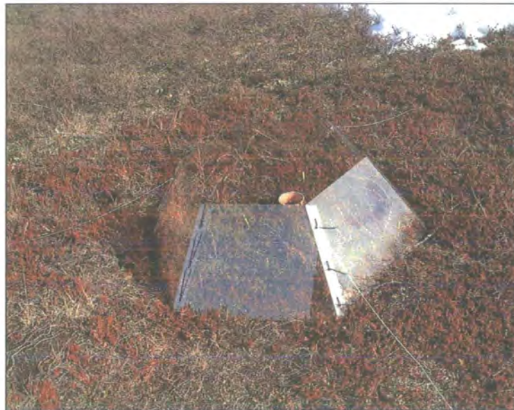
Figure 2.4: An example of an open-top chamber in the lower tundra site. The OTC had an area of 1\text{ m}^2 at the base and reached approximately 50 cm off the surface of the ground. The OTCs were secured with guy ropes to prevent movement. Photograph taken April 2003.
