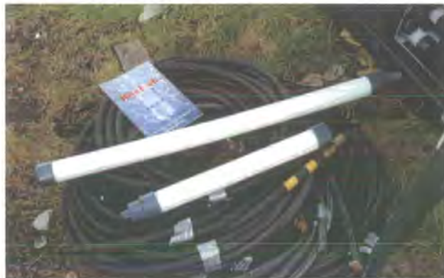
Figure 2-23 Diffuser Tubes & Airlines
