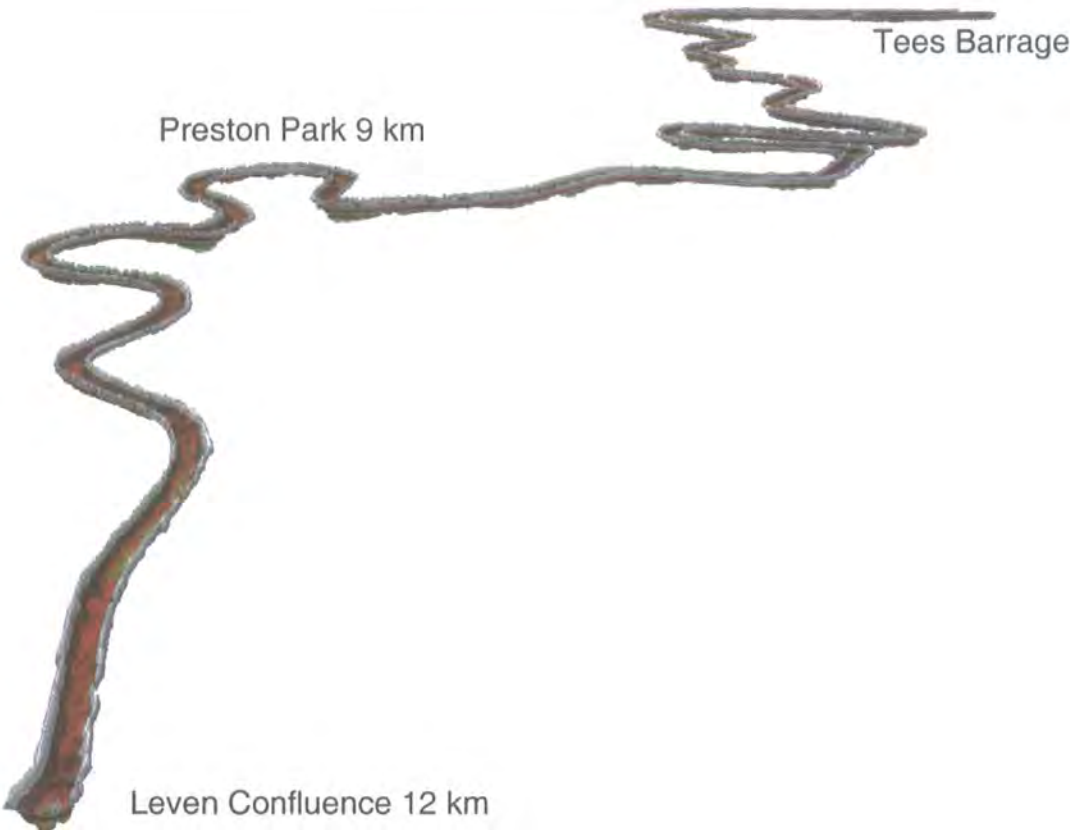
Figure 5-26 3-D model of the River Tees bathymetry from the barrage to Leven confluence (unscaled schematic)
