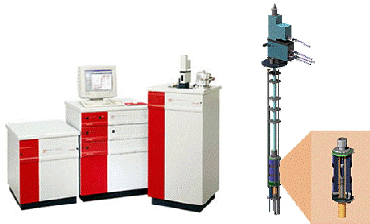
Fig 2.13: The MPMS5 SQUID magnetometer: schematic diagram of MPMS probe with blow up of superconducting solenoid detector coil (right). 24
