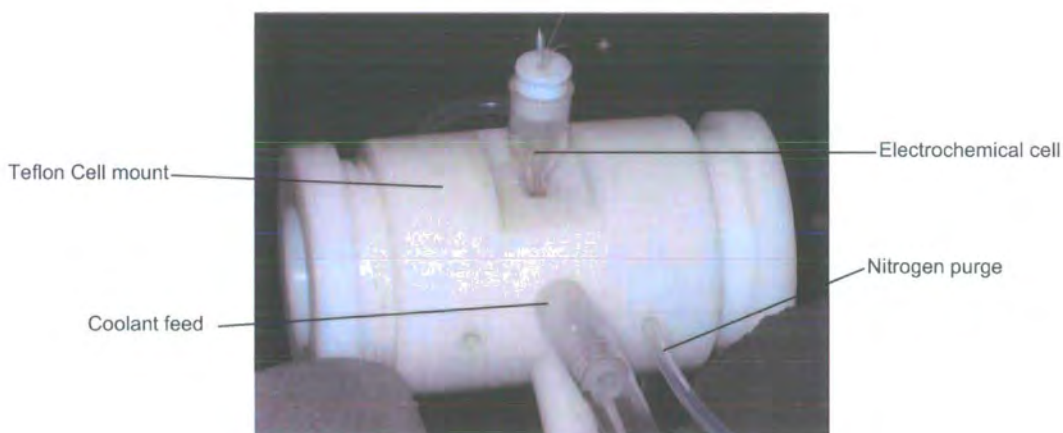
Figure 2.5. Spectro-electrochemical apparatus for UV-vis-NIR measurements
