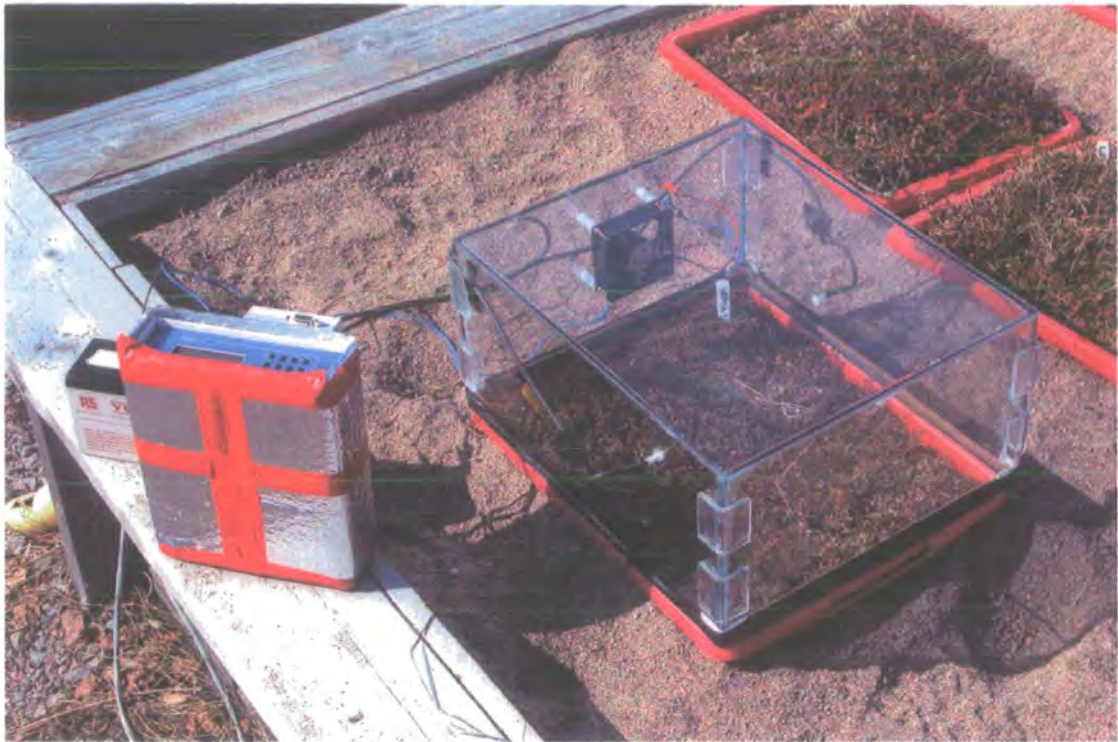
Figure 3-9: Monolith CO 2 exchange measurement; May, 2004.
