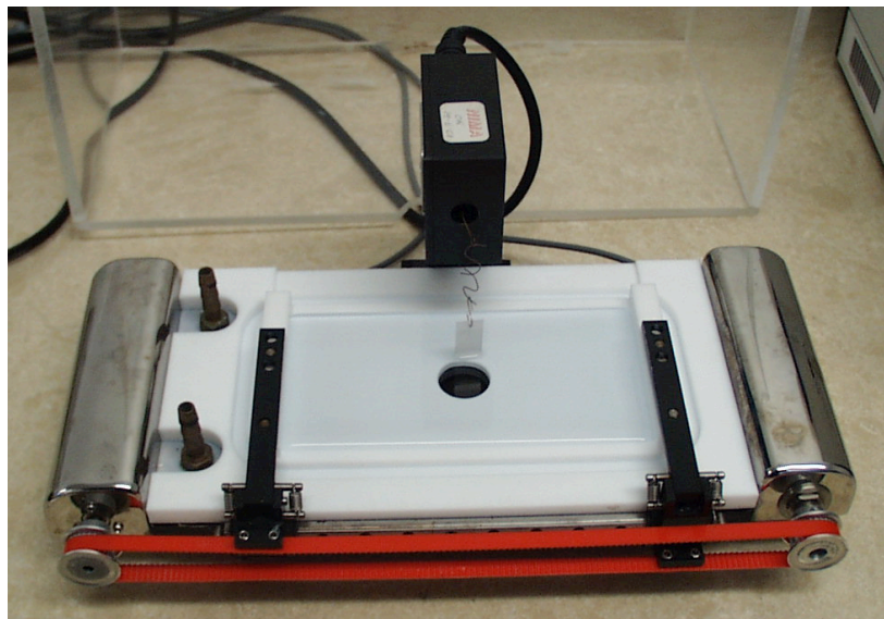
Figure 3.5: Photograph of the Langmuir trough (Nima Technology) used to carry out the work described in this chapter.
