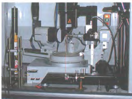
Figure 2.8: Picture of the SMART-CCD 1000 with the red laser. The thin red line gives an idea of the beam path.
