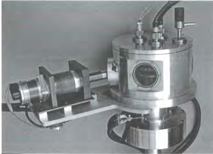
Figure 4.1. The top end of the strain probe, with the computer-controlled stepper motor (on the left).
