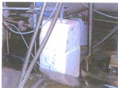
Fig 7 (cover the trap by a polystyrene box)
