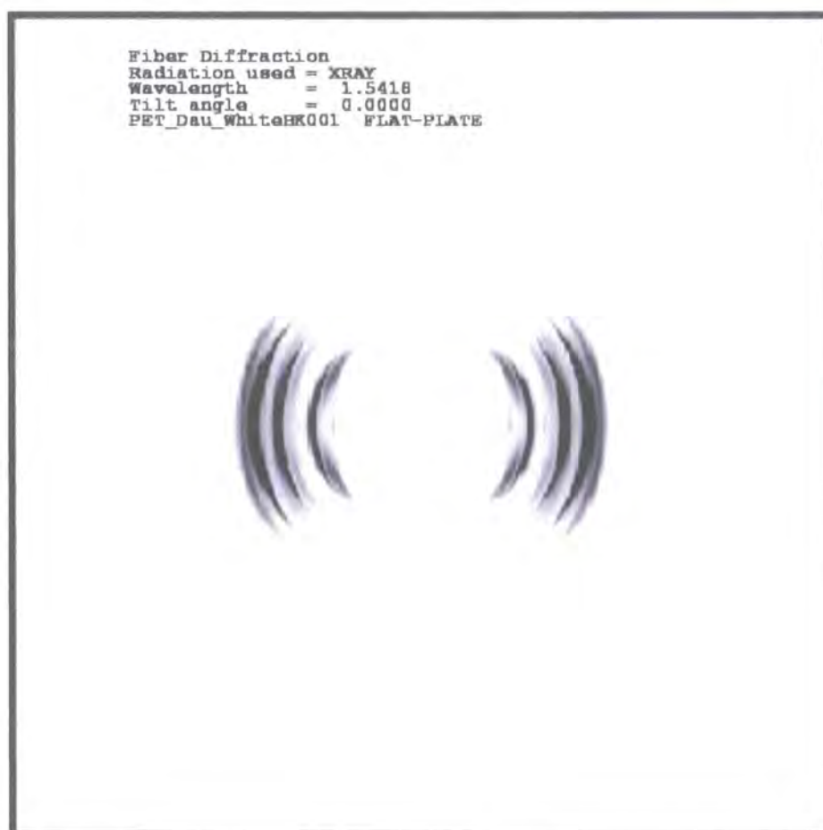
Figure 5-3: A simulated X-ray 'fibre' diffraction from oriented PET crystals
