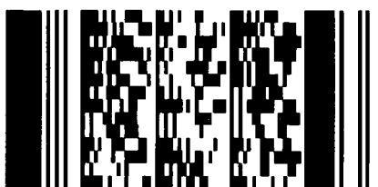
Figure 7: Stacked barcode example (PDF417)
