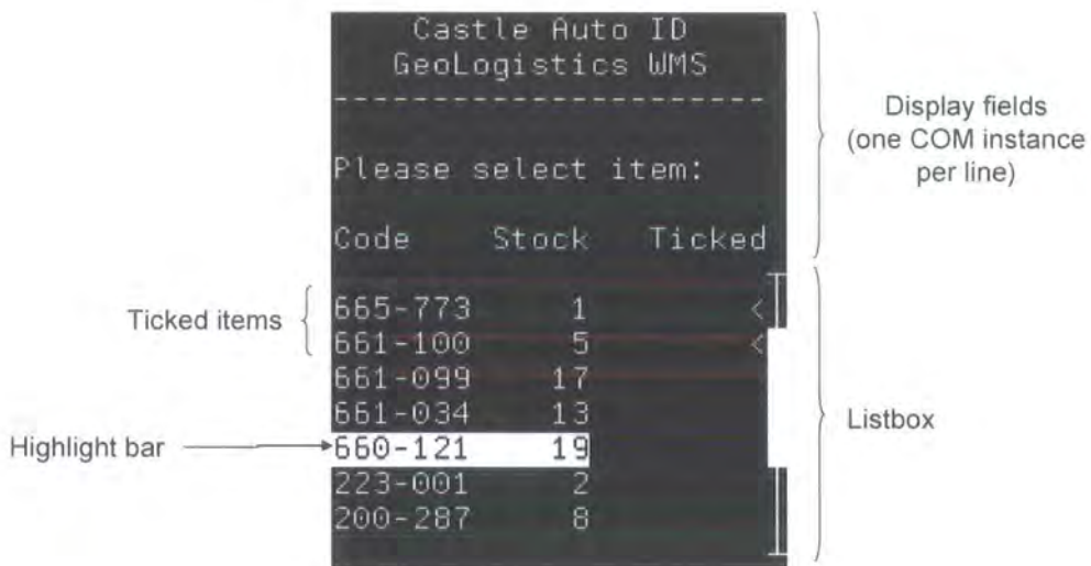
Figure 48: VT COM Server annotated in WMS screen
