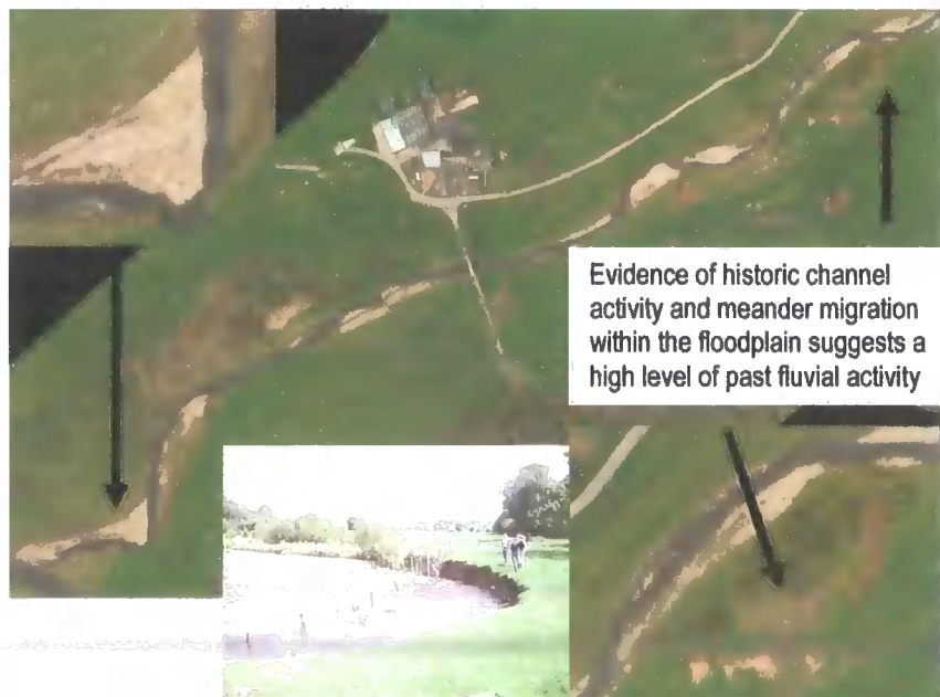
Figure 4.3: Demonstration of bank erosion assessment using aerial photographs where the primary cause is related to fluvial processes and sediment regime.
