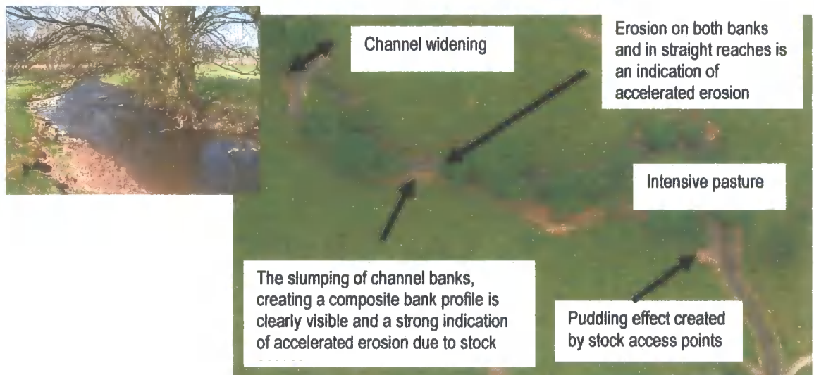
Figure 4.2: Demonstration of bank erosion assessment using aerial photographs where the primary cause of erosion is intensive grazing
