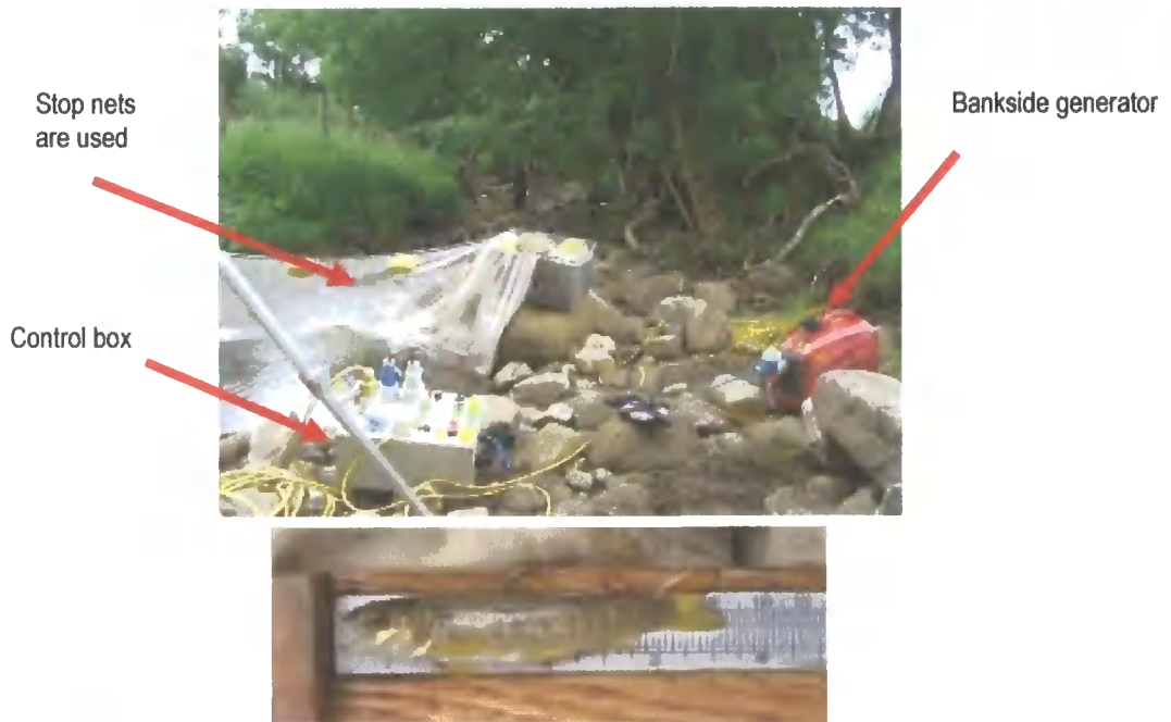
Figure 3.4: Quantitative electrofishing in action, using stop-nets and bankside generator-driven gear. Photographs courtesy of J. Brown.
