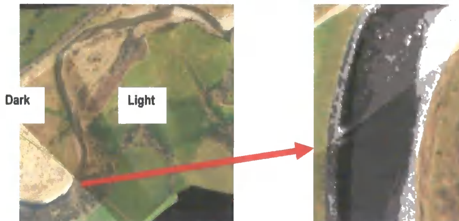
Figure 4.9: Illumination variations between images lead to error in the classification of water depth.
