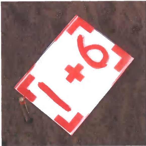
Figure 2.8 Panel used for ground control points (GCPs)
