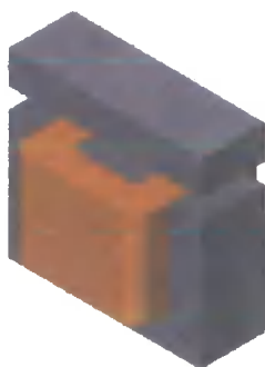
Figure 4.18 - Single E-core System
