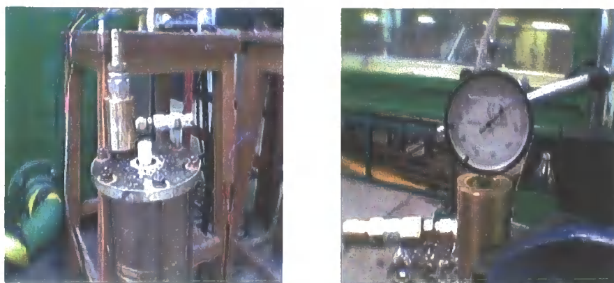
Figure 4.59 – Piston and Chamber (left) and Stroke Length Measuring (right)
