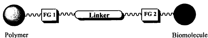
Figure 1.8. A representative structure typical of the proposed hetero-bifunctional linker conjugated system
