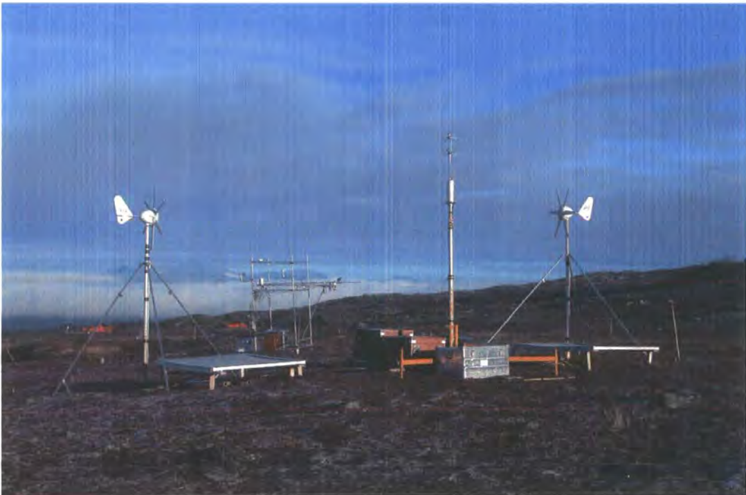
Figure 3-8: Automatic Weather Station and Eddy Correlation Tower deployed at the study site.
