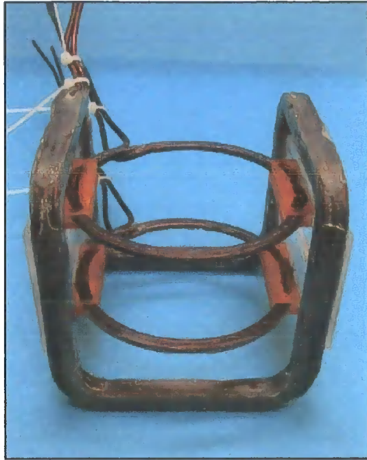
Figure 5.9. Photograph of the completed Baseball Lens. The Bias Coil pair was set within the Baseball Coil, using Araldite 2011 epoxy, to form the completed Baseball Lens. The white flecks that can be seen on the coil are places where excess epoxy was filed gently away.
