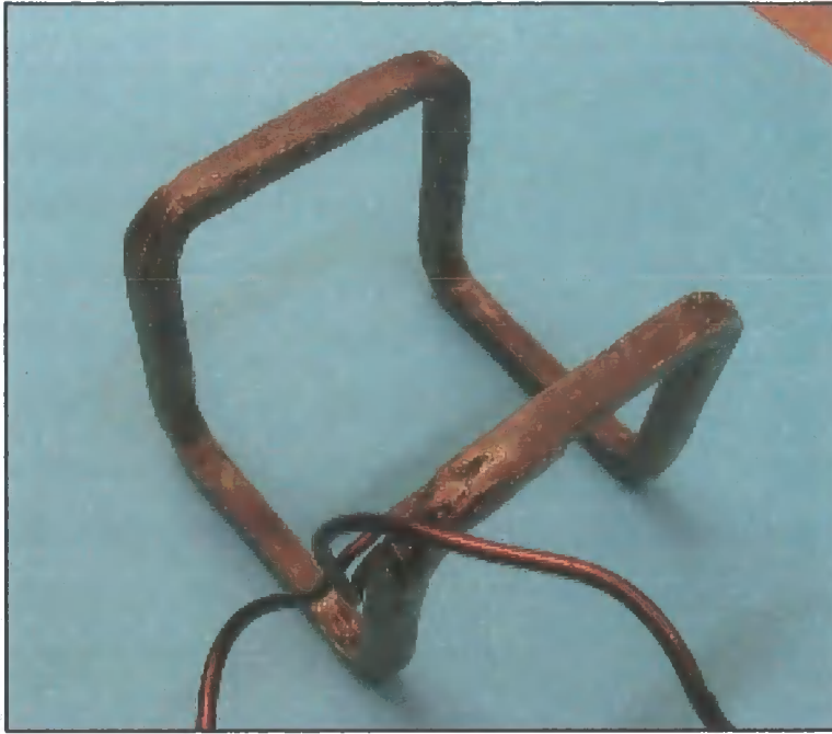
Figure 5.6. Photograph of the completed Baseball Coil. After the ninth turn was completed and set, the whole coil was coated in epoxy to provide extra rigidity.
