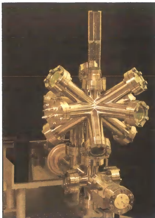
Figure 2.15. Photograph of the vacuum chamber detailed in the schematic in Figure 2.14. The main feature of the system is the specially commissioned 12-way cross, which has ports at specific angles for the purpose of a Moving Molasses phase in the experiment (see section 2.2).
