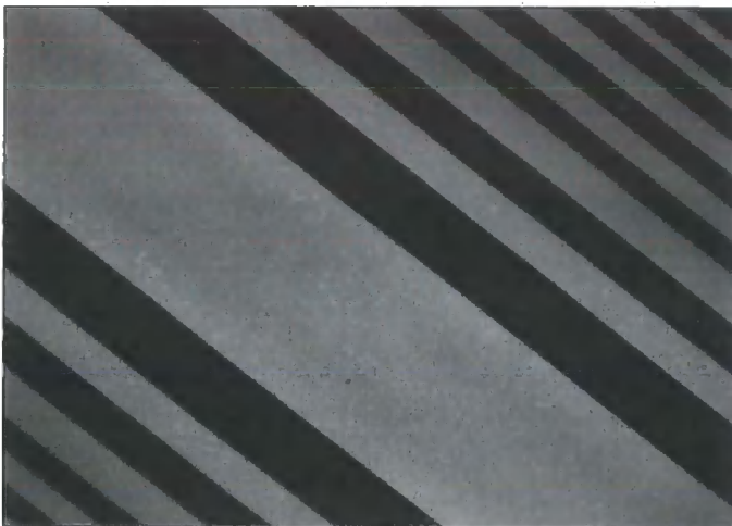
Figure 3.36: A CGH photo-reduced x25 from a laser-plotted master
