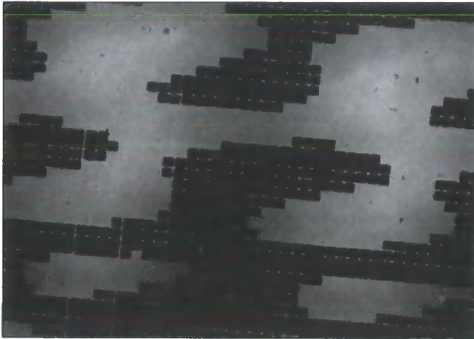
Figure 3.35: A CGH plotted using a laser writing tool
