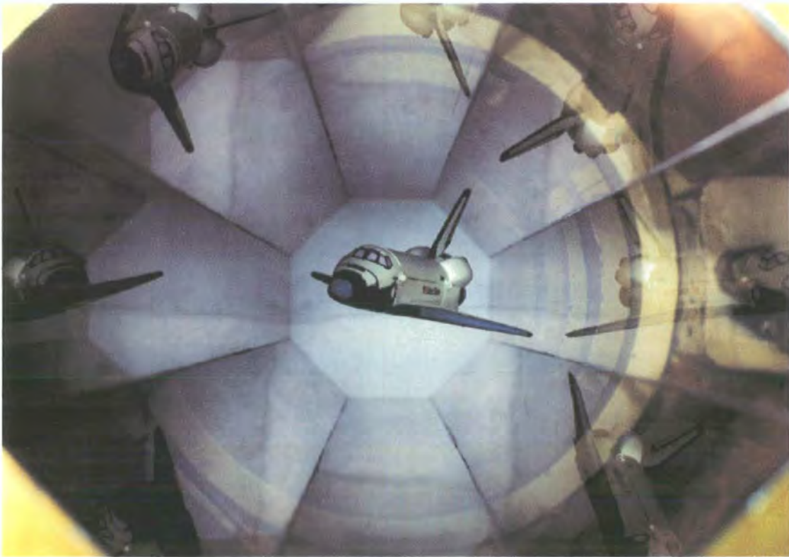
Figure 1.3.1, NASA's MSBS 158mm Wind Tunnel (NASA 1991) showing reflection of test vehicle in mirrored walls.
