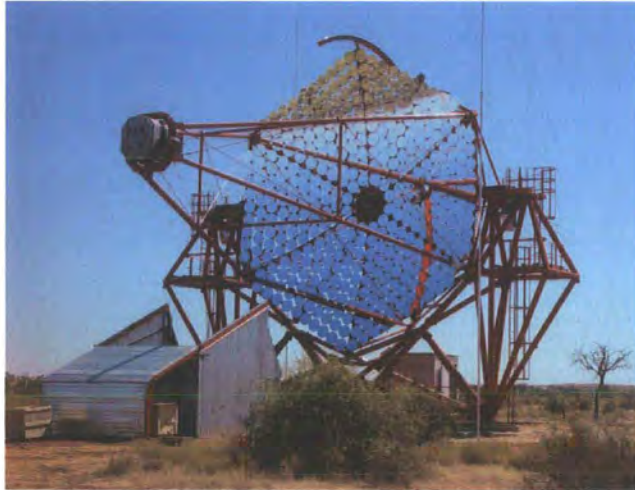
Figure 4.28: (from [331]) The first H.E.S.S. telescope. Each mirror element is 60 cm in diameter.
