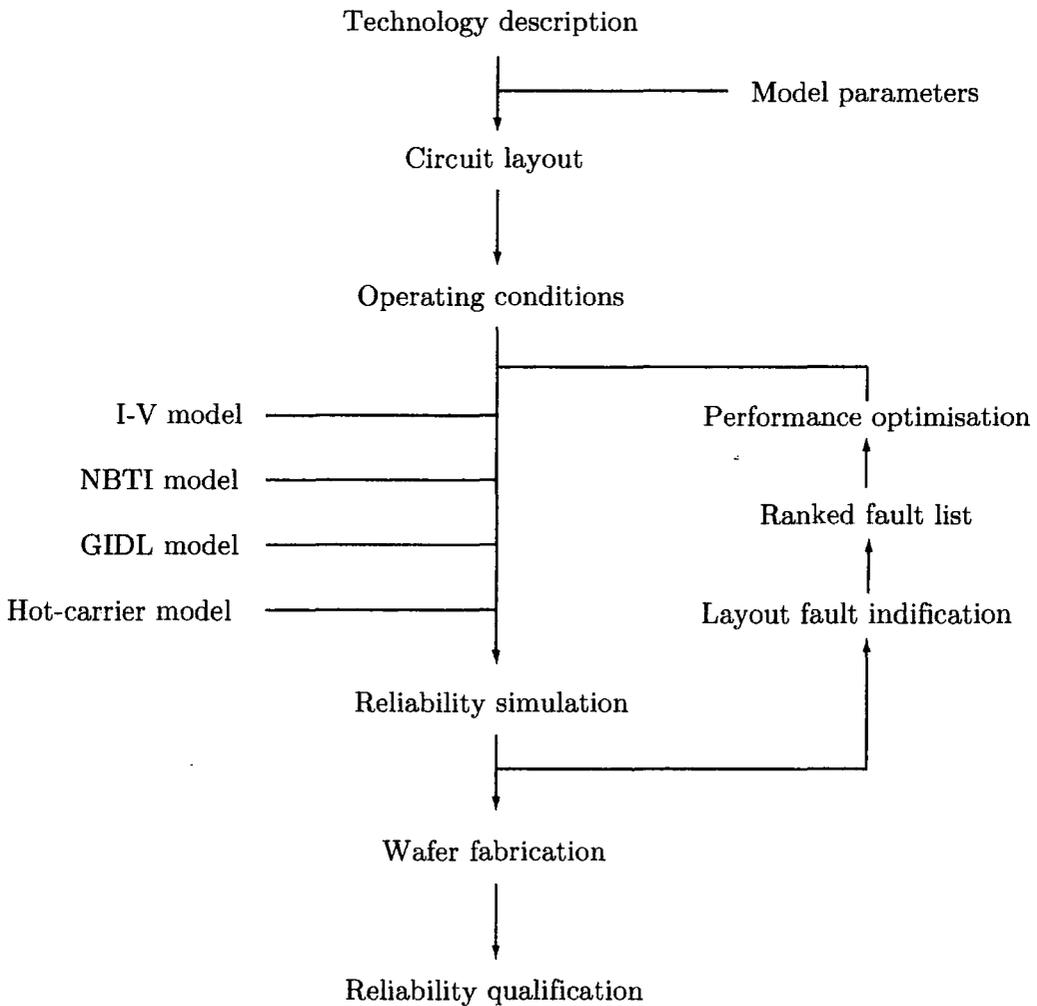
Figure 8.1: Development of methodology for layout diagnostics
