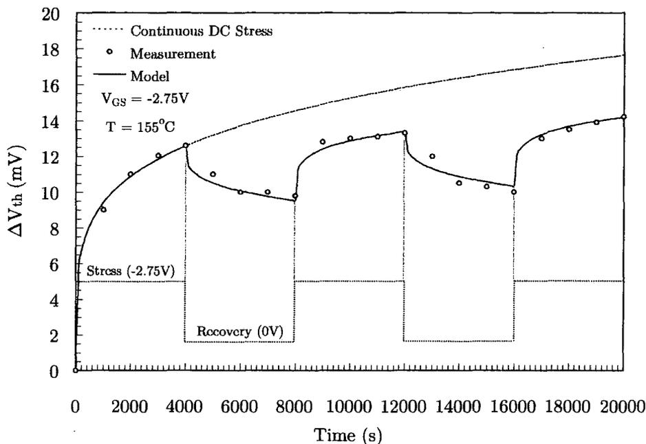
Figure 4.12: NBTI lock-in illustration
