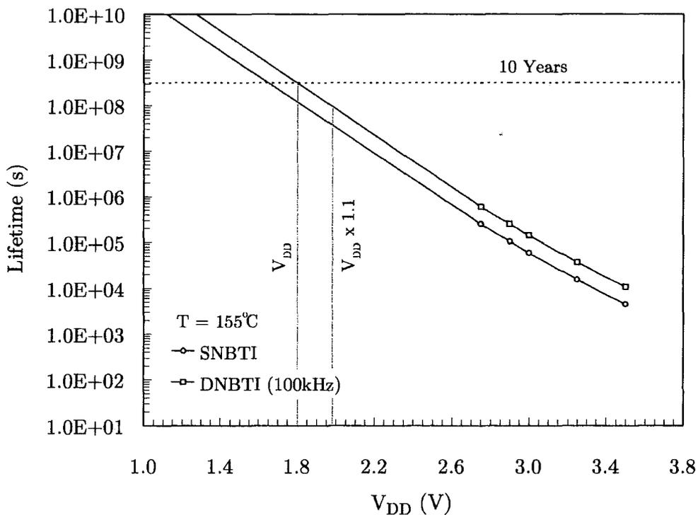
Figure 4.16: NBTI lifetime comparison
