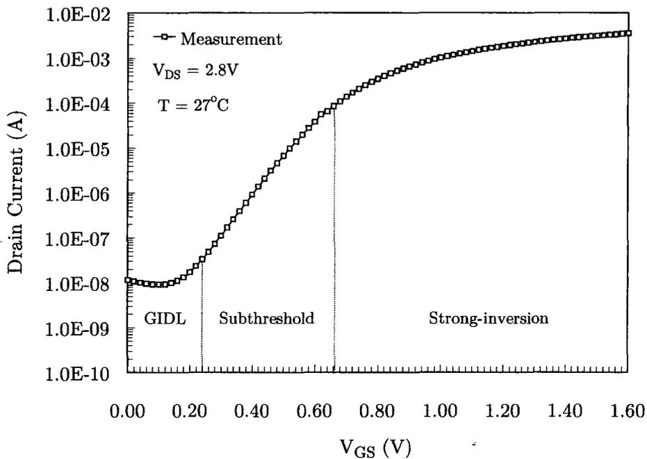
Figure 5.11: Illustration of device operating regions (n-channel)
