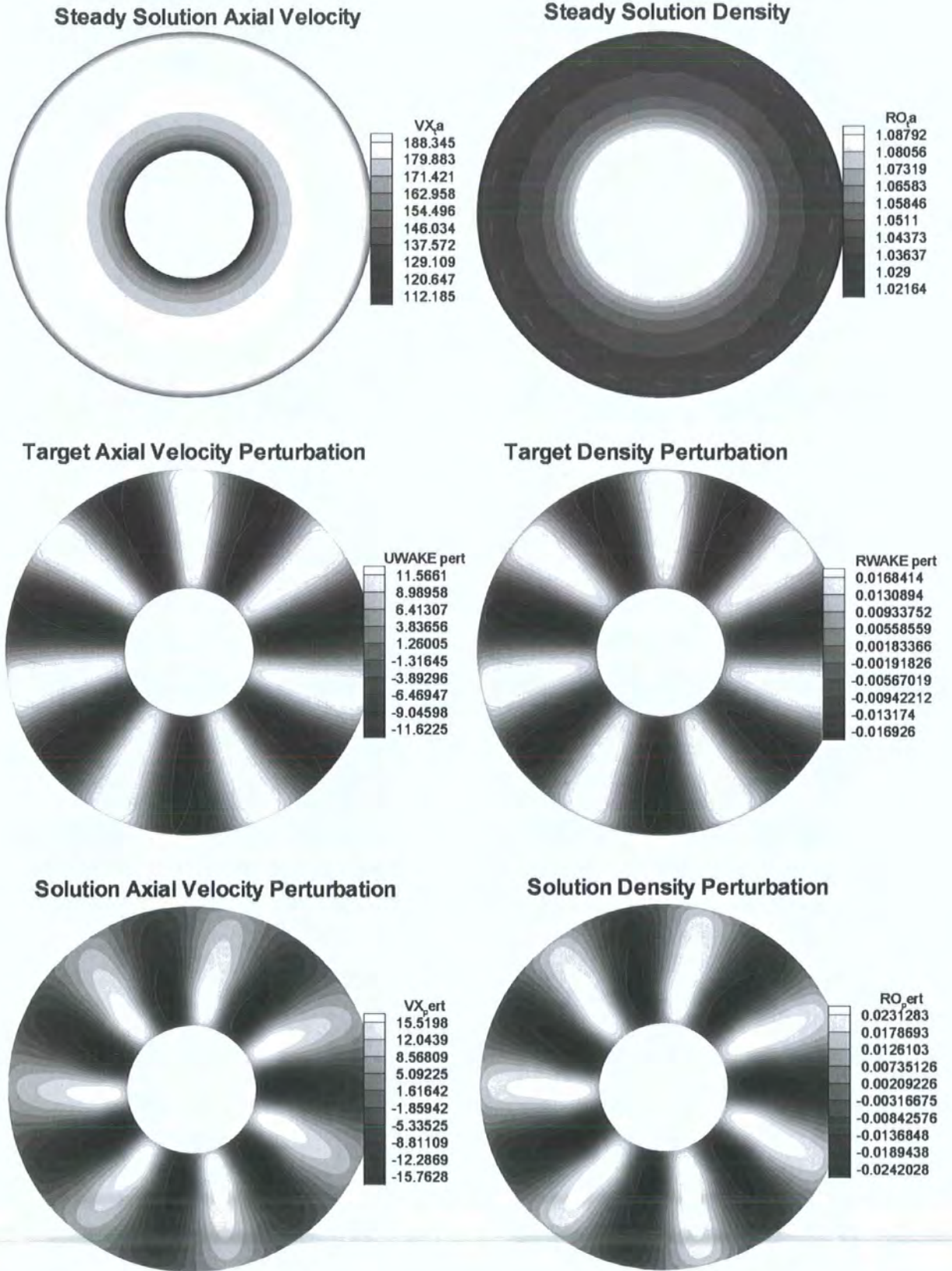
Figure 5.6: Inlet axial velocity and density distortion
