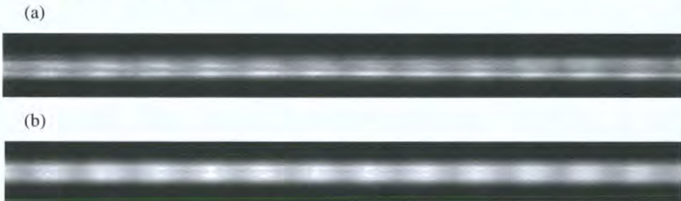
Figure 7.11 – (a) An un-agitated spectrum, (b) Agitated spectrum. Both taken within a few seconds of each other. A very slow input focal ratio, with attendant very low S/N_M , is shown since the modal noise along the slit in the un-agitated case can actually be seen by eye, even with partially coherent illumination. The beating along the spectrum is due to the laser filter.
