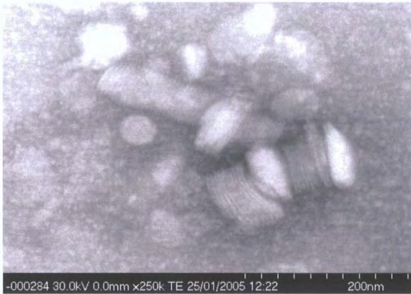
Figure III.2.19. TEM images of stacked planar structures obtained after a two fold increase in the dialysis rate.
