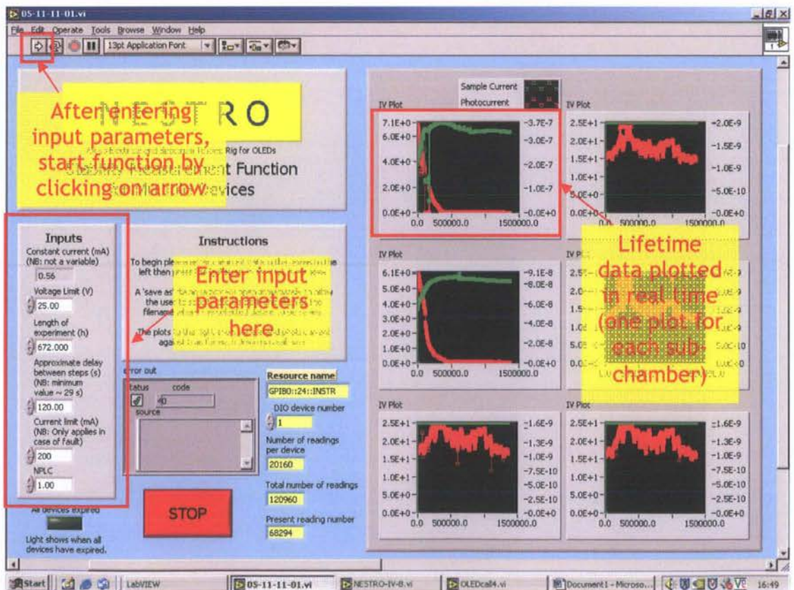
Figure 4 Screen grab of virtual instrument for constant current stability characterisation
